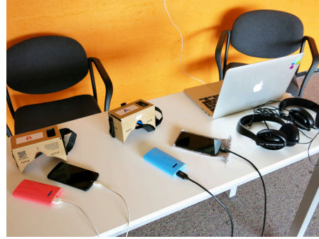
(b) Photo of the testing equipment used in this study: Two Google Cardboards , two smartphones with external batteries, two headphones, and laptop running the game server.
